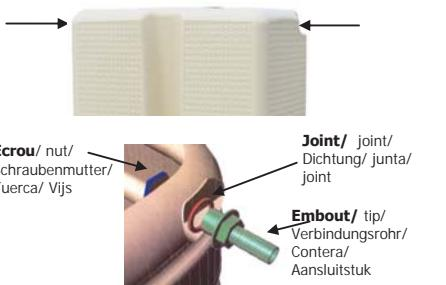
1/ Bore the hole of filling (materialised on the tank) on the adequate side and refine it taking away burrs. Then connect the connecting tips on the tank.
