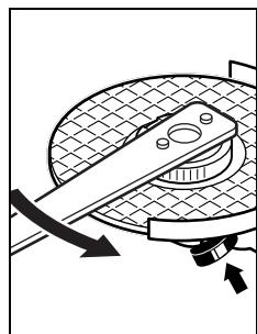
A properly fastened, undamaged quick-clamping nut can be manually loosened by turning the knurled ring in anticlockwise direction.
