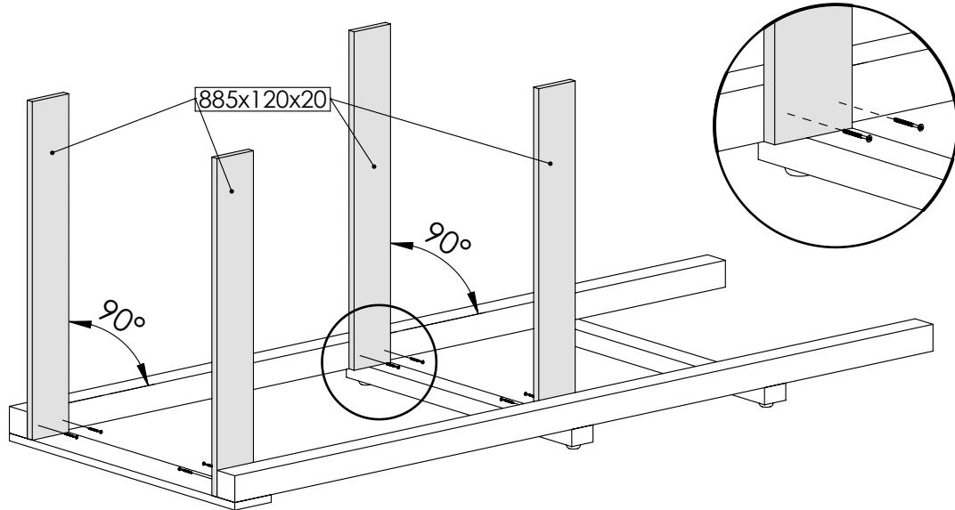
**4** $\varnothing 4 \times 50\text{mm}$ B<sub>x8</sub>
