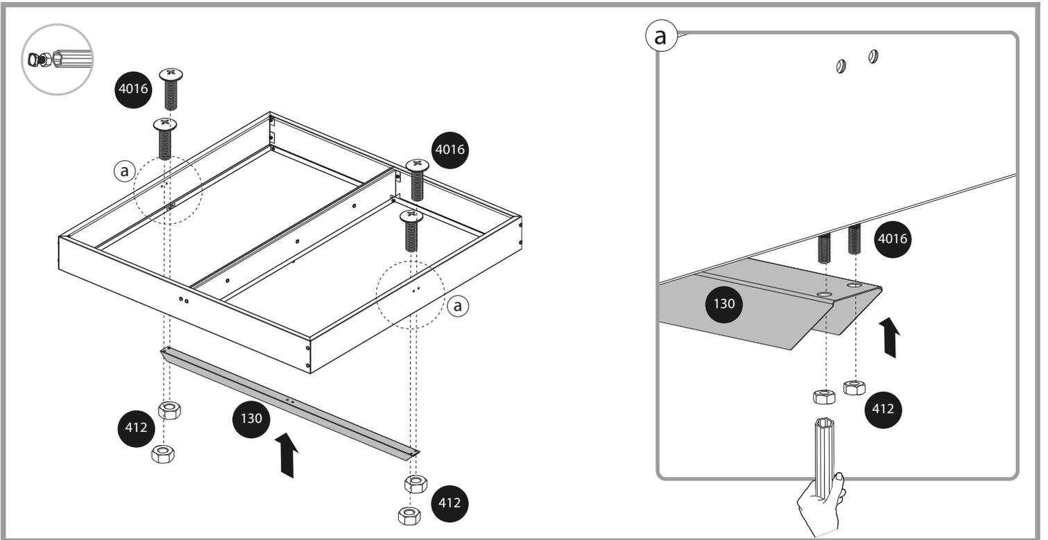
The diagram illustrates the assembly of a rectangular frame. A long thin bar (130) is being attached to the bottom edge of the frame. Four screws (4016) are used to secure the bar to the frame's side rails. Four nuts (412) are used to secure the screws. Callout 'a' indicates the connection points. A hand is shown holding a screw (4016) to be inserted into the frame.
