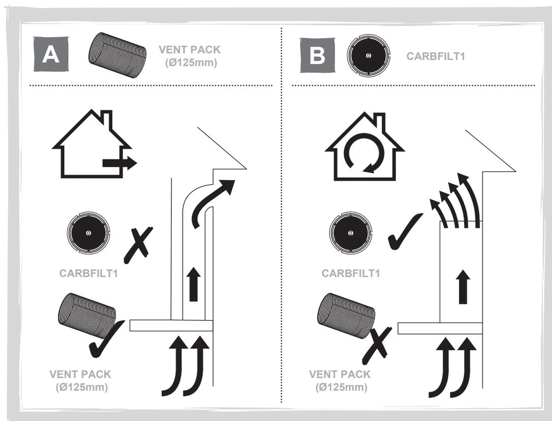
**EN** Choose a type of installation: Ducted option **A** (extraction to the outside) or Recirculation option **B** (no extraction to the outside). This appliance is for installation to a wall or under a cupboard bridging unit.
