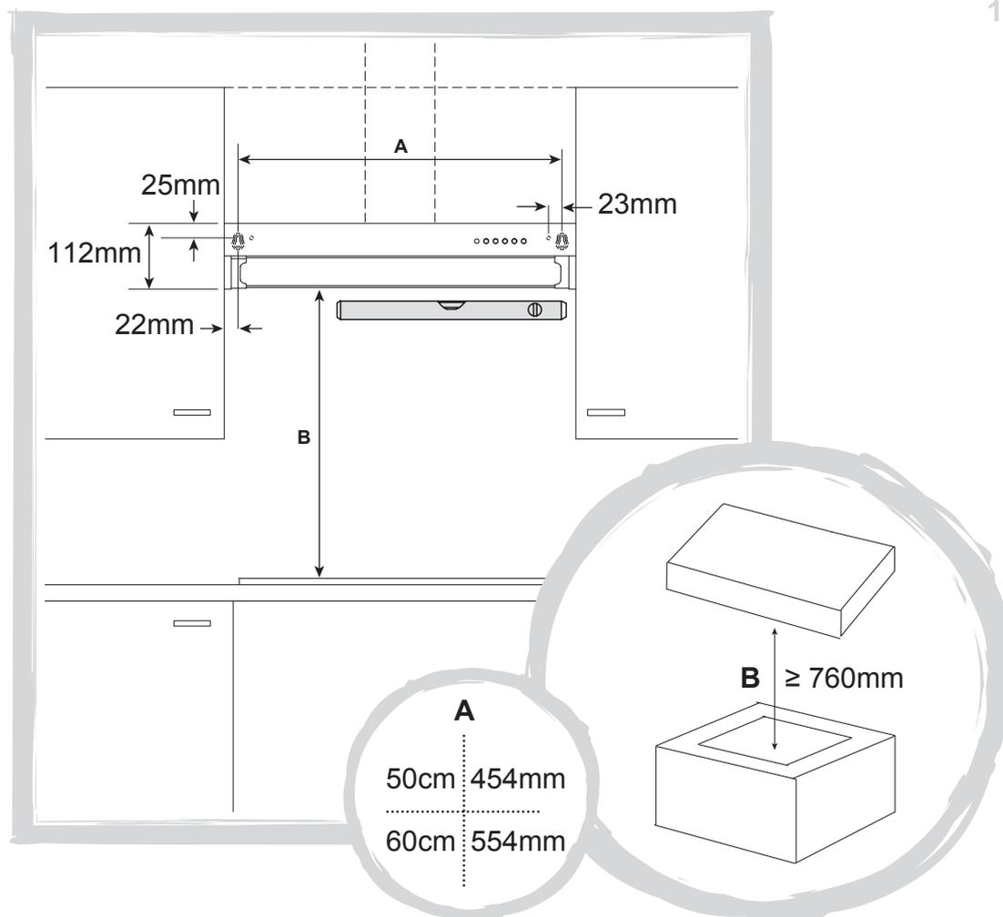
EN Mark the wall with the 4 hole positions as shown in the diagram. Please ensure you use wall fixings appropriate to the substrate this appliance will be fixed to, for example, solid wall fixings.
