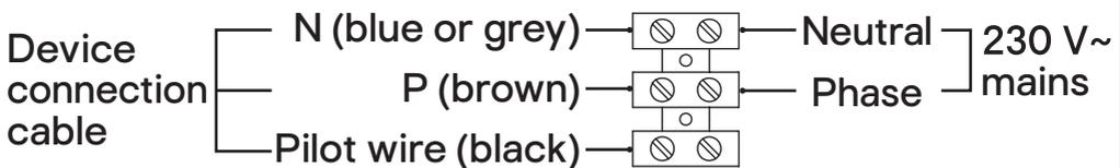
**Note:** The programming orders are transmitted by the above signals, measured in relation to neutral.
