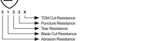
The pictogram above shows that this glove protects against Mechanical Risks as per EN388:2016. The numbers indicate performance level. X: indicates the glove falls below the minimum performance level for the given individual hazard.
