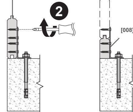
**EN** Laying on concrete slabs (not included)
