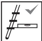
EN Leaning ladders with steps shall be used that the steps are in a horizontal position.
