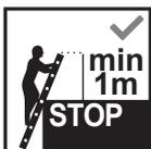
EN Ladders used for access to a higher level shall be extended at least 1m above the landing point and secured, if necessary.
