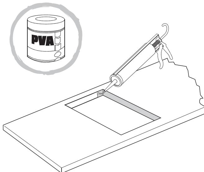
➊ Seal the cut edge of the worktop using silicone sealant or PVA adhesive.
