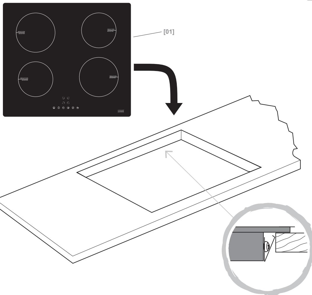
**EN** Once the worktop edge has cured, and the tape is fitted, position the hob into the cutout in the worktop. Apply gentle downwards pressure onto the hob to push it into the worktop ensuring a good seal around the outer edge.
