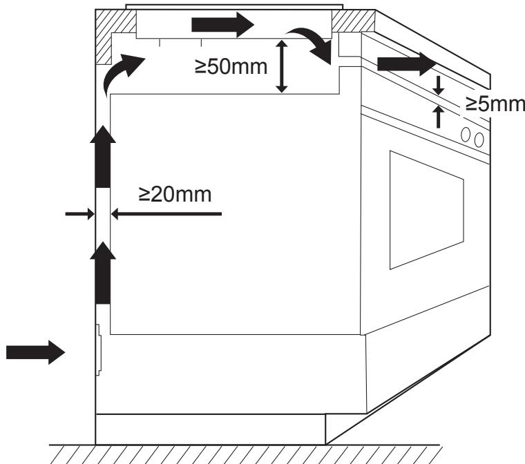
**EN** The induction hob must be well ventilated and the air inlet and outlet must not be blocked. Ensure you select a heat-resistant work surface to mount the induction hob.
