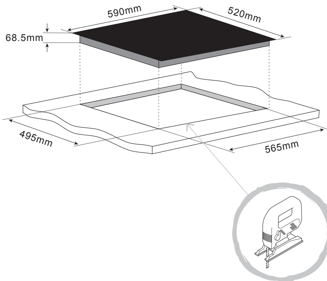
**EN** Cut an aperture in the worktop using a jigsaw as shown. The worktop should be at least 30mm thick and made of a heat resistant material.
