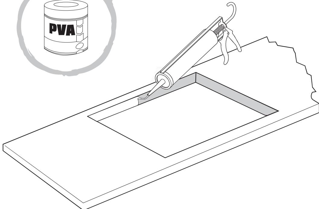
**EN** Seal the cut edge of the worktop using silicone sealant or PVA adhesive.
