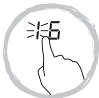
5. Set the tens of minutes by touching the slider control (e.g. 9) and the timer is set at 96 minutes.
