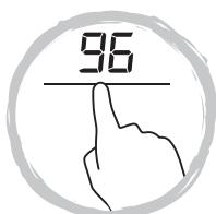
6. Buzzer will beep for 30 seconds and the timer indicator shows “00” when the setting time finished.
