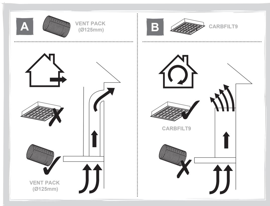
EN Choose a type of installation: Ducted option **A** (extraction to the outside) or Recirculation option **B** (no extraction to the outside). This appliance is for installation under a cupboard bridging unit only.
