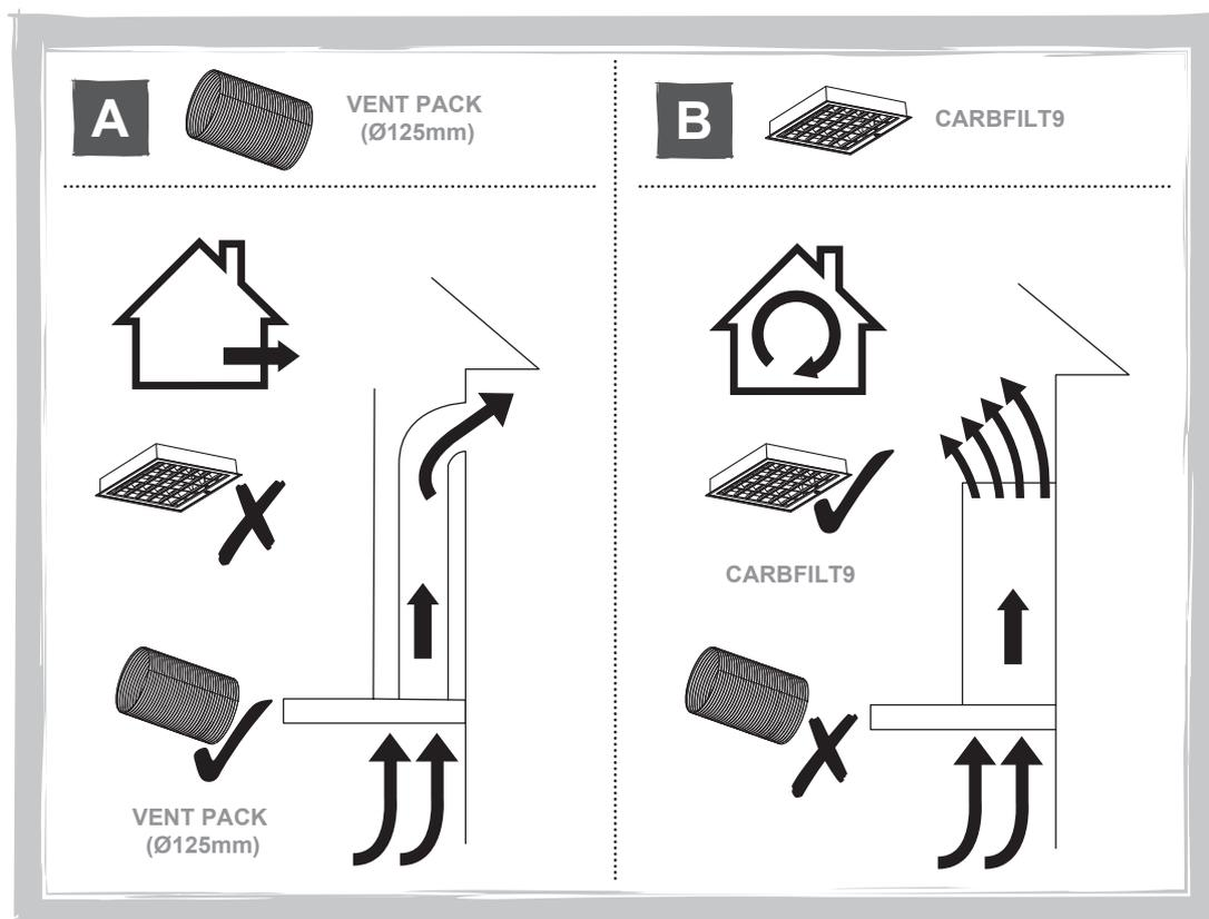
**EN** Choose a type of installation: Ducted option **A** (extraction to the outside) or Recirculation option **B** (no extraction to the outside). This product is for mounting in a wall bridging unit.
