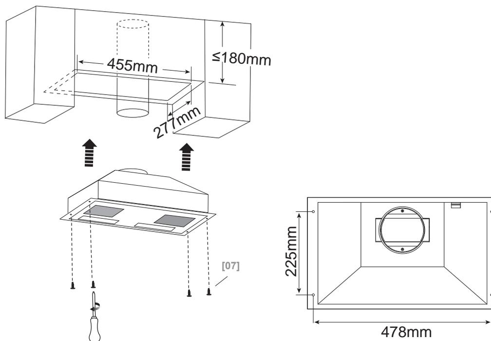
EN Mark 4 holes as per the diagram above. Using the dimensions in the diagram, cut an aperture in the base of the bridging unit using a jigsaw. Secure the hood into the aperture using the 4 screws provided.
