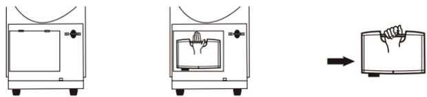
Unscrew the central screw and remove the trap door hiding the water tank.
