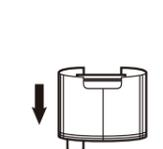
Screw the cap back and put the water tank in the original position in the fan then screw back the trap door.
