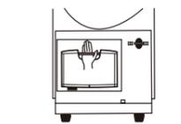
Remove the foam protection and remove the water tank by holding it.
