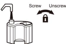
Unscrew the cap of the water tank and add 50% tap water and 50% demineralised (deionised) water in order to reduce the impact of the scale.
