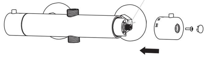
**EN**  This mixer has been set in the factory with balanced pressures and hot water supply at 65°C. When your operating conditions vary significantly from the above, the temperature of the mixed water may vary from the setting. If this is the case, you can set the temperature of the mixer to suit your requirements.
