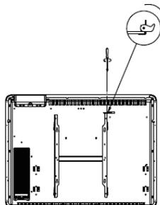
2-Position the wall mount in the desired location. Use a spirit level to ensure that it is horizontal. Mark the location of the 4 screws to be used to fix the wall. Drill holes in the wall to attach the appropriate anchoring system. Attach the bracket to the wall.
