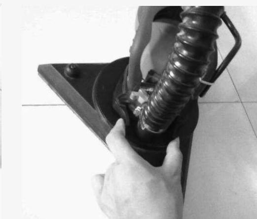
c. Press the two small clamp block , to make the sanding pad take off when need to change another pad
