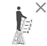
Do not stand on the 4 top rungs of a combination ladder
