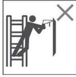
Avoid work that imposes a sideways load on ladders, such as side-on drilling through solid materials
