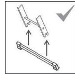
The ladder must only be used with installed crossbars
