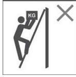
Do not carry equipment which is heavy or difficult to handle while using a ladder
