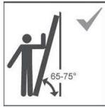
Leaning ladders with rungs shall be used at the correct angle
