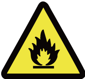
Caution, risk of fire, R290
