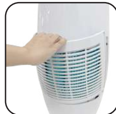
Hold the unit firmly and grasp only the top center of the dust filter then pull it out hardly in one time (see above image).
