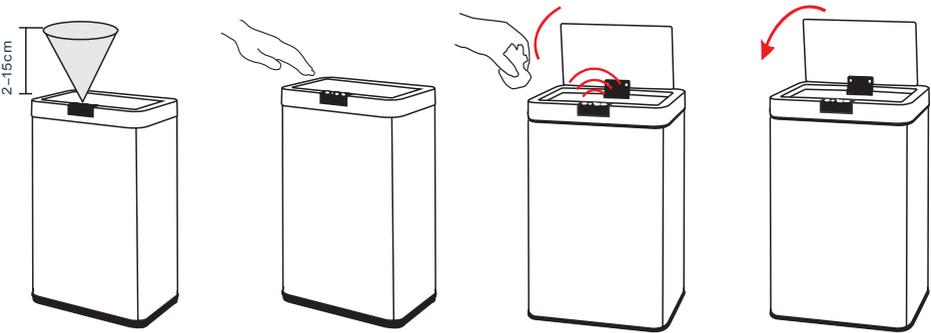
SENSOR ZONE is above 2-15cm above the sensor panel
