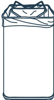
STEP 2 : Place the plastic bag bracket on the top of the can body. The surplus will be folded up inside the can.
