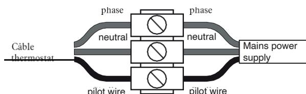
Case 1: User electrical system without pilot wire: the pilot wire (black) must not be connected. If your installation does not have a pilot wire, this wire must not be connected. Never use the earth wire of your installation (yellow-green colour) to connect this pilot wire. If there is no pilot wire, insulate the stripped end of the black wire to avoid any electrical contact with the other wires or the earth.
