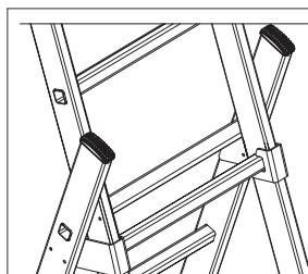
Let the middle section slide upwards, until the last rung is positioned on the level joint. Then open the ladder in double position.
