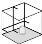
Release the transport restraint, push the slide switch (3) to the left. The laser lines can be switched individually with the selection button.
