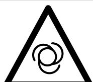
Warning! The unit is equipped with an automatic start control. Keep others away from the work area of the device!
