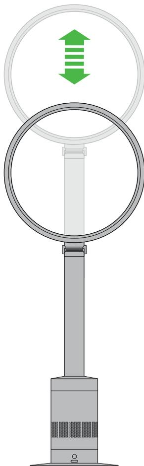
Carefully hold the base and the top of the air loop amplifier. Tilt forward or backward for the required airflow angle.
