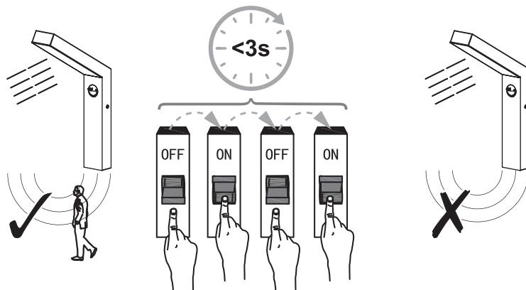
**EN** Deactivate motion sensor and keep light on
