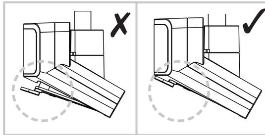
**EN CAUTION:** Cover must be closed completely for water ingress protection.
