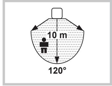
**EN** To set a desired product setting (Time, Lux sensibility or sensor range) keep adjusting the corresponding knob until the lamp lights up.
