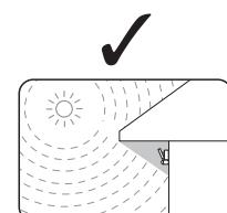
**EN** Avoid sunlight falling onto the lens of sensor
