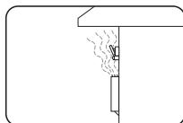
**EN** Avoid installing around the heat sources (ie. Air vents, heater...)
