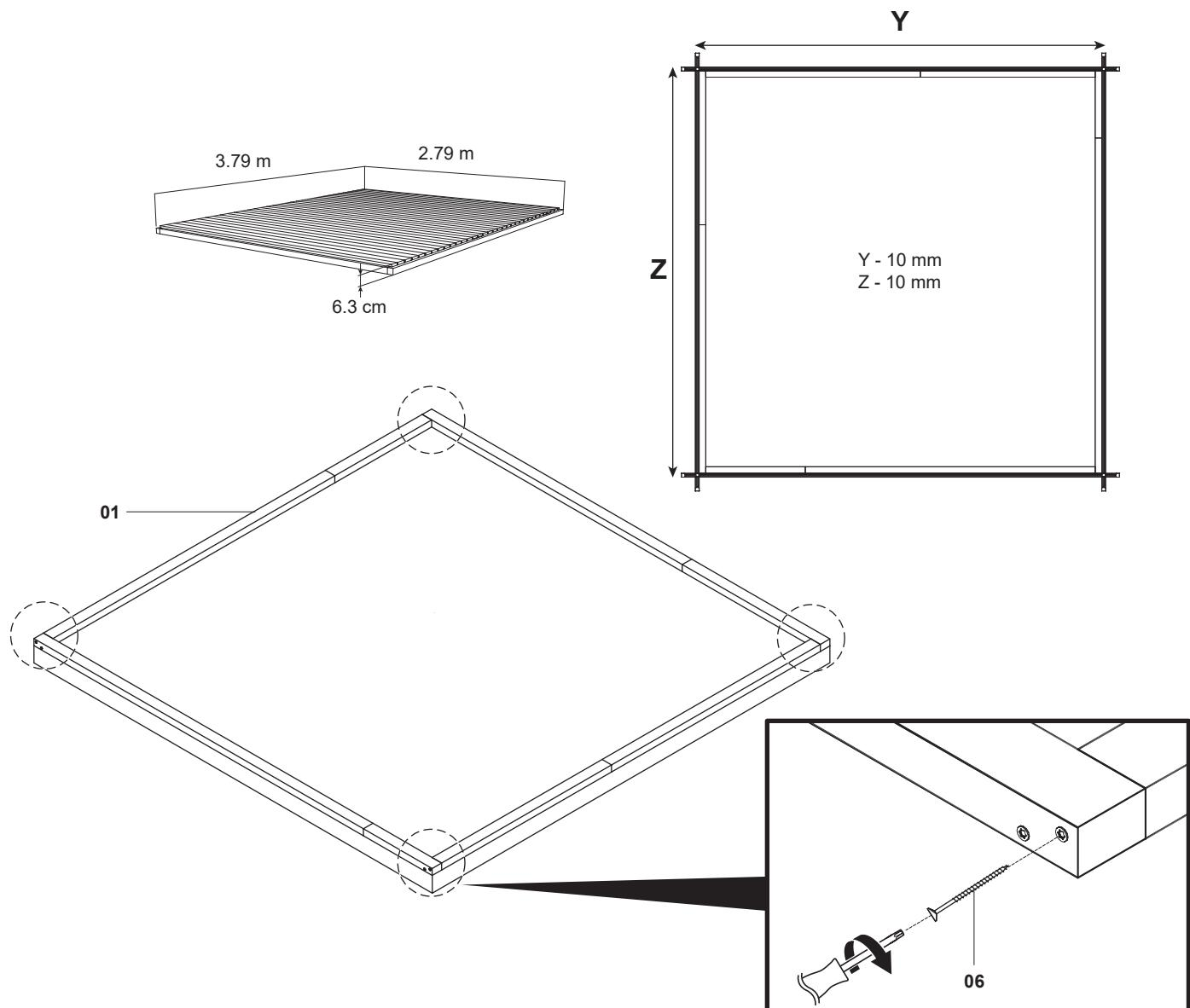
**EN** Laying on concrete slabs (not included)
