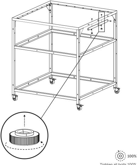
Tighten all bolts 100% **DO NOT** over tighten bolts
