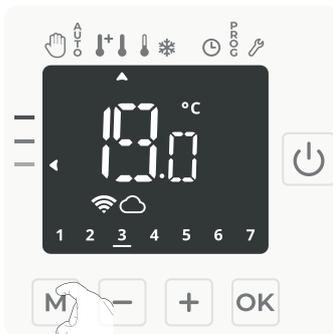
2- Once the mode is selected, adjust the desired setting temperature with **-** or **+**. The modified value is saved automatically.
