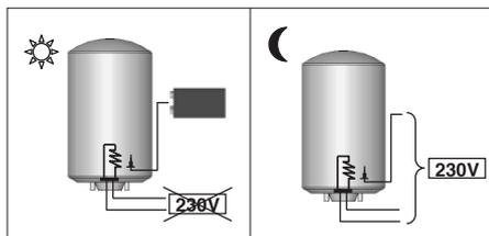
Figure 13 - PROfessional TECH alimentation de nuit + batteries
