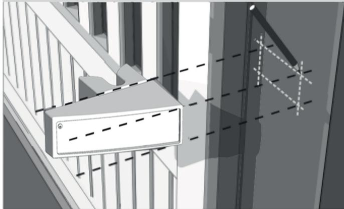
VEUILLEZ FERMER LE PORTAIL EN LE CENTRANT ENTRE LES PILLIERS. LE PORTAIL DOIT COUVRIR LE PILLIER D'ENVIRON 3CM. A L'AIDE DU GALET DE RECENTRAGE, PLACEZ LE SUPPORT ET TRACEZ L'EMPLACEMENT DES FIXATIONS.
