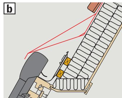
**ENGLISH:** As a precondition to avoiding any damage to the roller shutter in very cold regions and in regions with heavy snowfall, either a snow-wedge or a snow stop must be installed above the roller shutter **[a], [b]**. The roller shutter is protected against overload, and will stop automatically if it is blocked.
