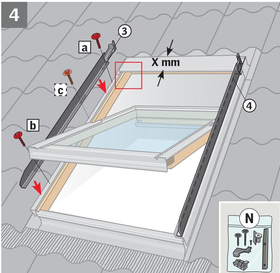
**ENGLISH:** Measure the width of the window top cover (**X mm**). Depending on this width place the roller shutter side covers as shown in the detailed drawings **A**, **B** or **C**. Fix roller shutter side covers with screws **a**, **b**, **c**. Fit screw **c** only if cover screw in this position was removed earlier, see ill. 3.
