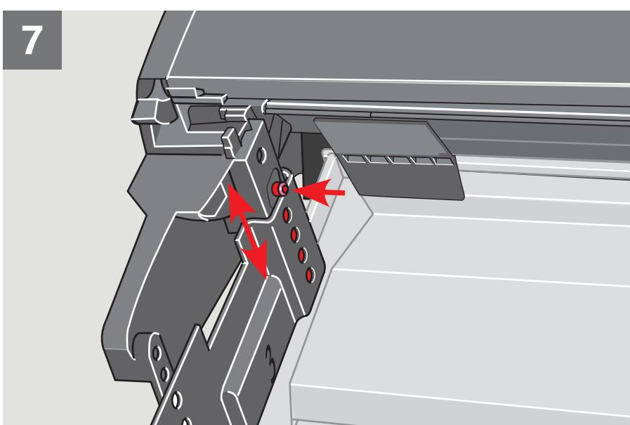
**ENGLISH:** Lower the roller shutter top casing as much as possible. Do **not** press the top casing against the roofing material **a**, **b**.
