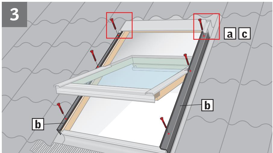
**ENGLISH:** Remove cover screws except the top cover screw **a**. The number of screws depends on the size and type of the window. Do **not** remove side frame covers **b**. If there is a mark at the top instead of a hole, drill hole through mark **c**. Place sealant on **all** screw holes **d**.
