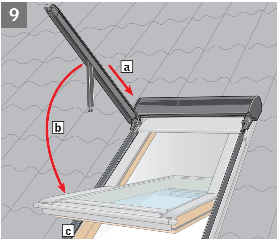
**ENGLISH:** Push side channels into position **a** and lay down on side covers **b**. Attach opening restrictors to side covers with screws **c**.
