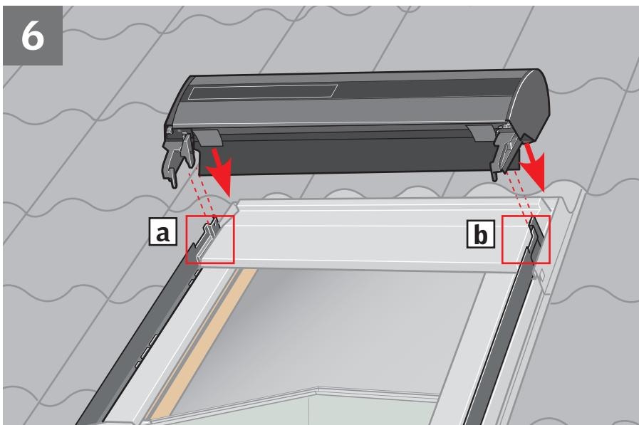
**ENGLISH:** Fit roller shutter top casing into grooves on side covers **a**. Check that rubber gasket at the back fits smoothly against outside of window **b**.
