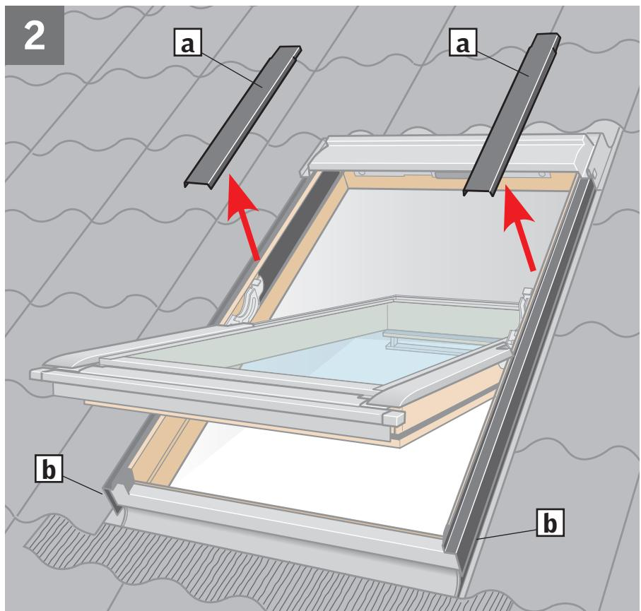
**ENGLISH:** Remove covers indicated temporarily by releasing the snap locks **a**. Note the position of the covers for later refitting. Do **not** remove side frame covers **b**. Drill hole through the marks in the side frame covers **c**. Place sealant on **all** screw holes **d**.
