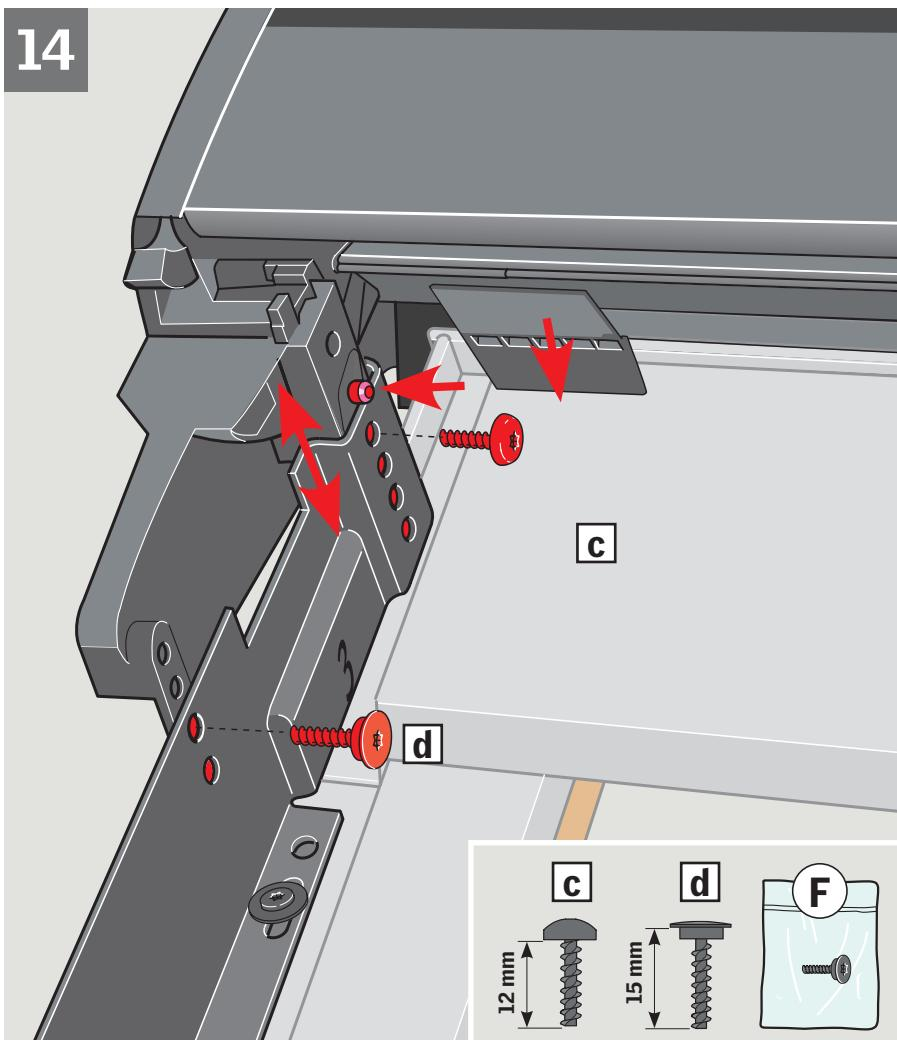
**ENGLISH:** Lower the roller shutter top casing as much as possible. Do **not** press the top casing against the roofing material **[a], [b]**. Fit securing screws after installing the roller shutter top casing **[c], [d]**.
