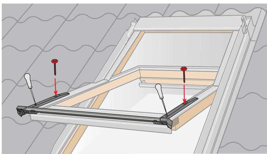
**ENGLISH:** Fit storm brackets and bottom cover temporarily with screws in the upper holes. Make a mark with bradawl through the lower holes.
