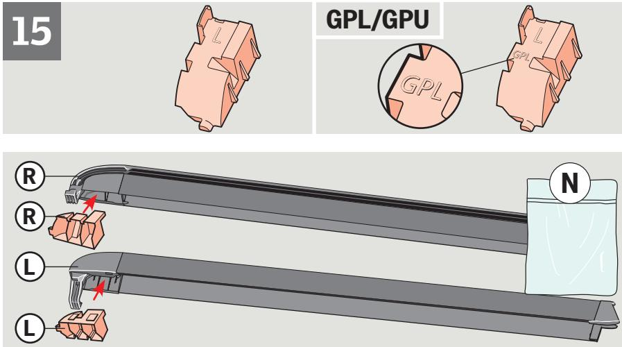
**ENGLISH:** Fit plastic insert pieces on the roller shutter side channels **[a], [b]**.
