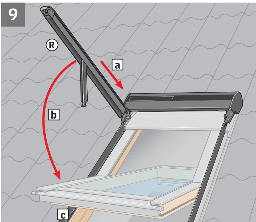
**ENGLISH:** Push side channels into position **a** and lay down on side covers **b**. Attach opening restrictors to side covers with screws **c**. The roller shutter is now ready for use. For important information, see pages 42-44. For operation of the roller shutter, see enclosed directions for use.
