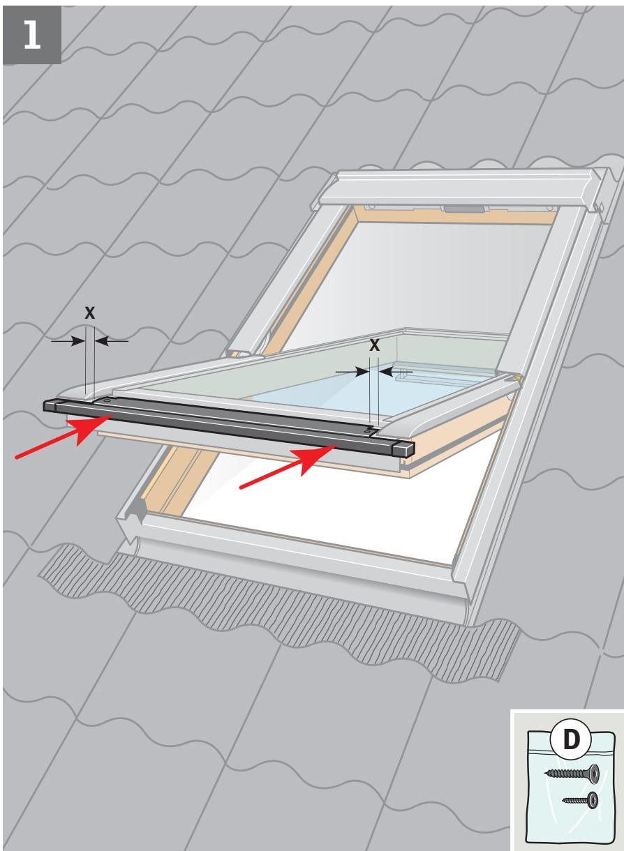
**ENGLISH:** Position bottom cover and push up against bottom edge of profile. Distance **X** must be the same at both sides. Make a mark with bradawl through holes in bottom cover **a**. Drill  $\varnothing 3$  mm holes **b**. Fit bottom cover **c**.
