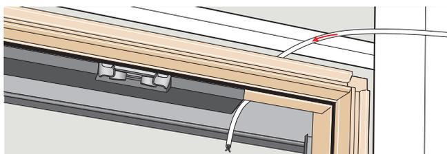
**ENGLISH:** Open window using handle (a). Pull the control bar downwards (b) and rotate the sash 180 degrees (c). Remove the insulation material in the top frame with a screwdriver (d). Break off the very end of the insulation material at the perforation (e). Refit the insulation material in the top frame (f). Lead the cable through the hole in the top frame and through the hole in the sash. Remove cover cap from sash, if any. Cut the cable to length leaving about 200 mm surplus (g).
