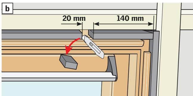
**ENGLISH:** Remove cover cap (a). If a frame insulation collar of installation set BDX is fitted around the window, the insulation material must be cut away from around the cover cap (b). The insulation material must be replaced after the wiring has been completed.
