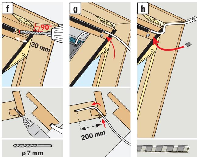
**ENGLISH:** Open window using handle (a). Pull the control bar downwards (b) and rotate the sash 180 degrees (c). Shorten rubber gasket (d). Set sash opening angle as shown (e). Maintain opening angle and drill hole at right angles to frame through the sash (f). Lead the cable through the hole and cut the cable to length leaving about 200 mm surplus (g). Place sealant around the hole. Fasten cable onto lining (h).
