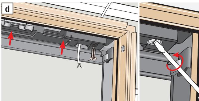
**ENGLISH:** Remove the insulation material in the top frame with a screwdriver (a). To make room for the cable, make a hole in the insulation material in the shown area with a bradawl (b). Lead the cable through the hole in the top frame and through the insulation material (c). Refit the insulation material in the top frame (d). Make sure to tighten the cable to avoid getting the cable caught between the insulation material and the top frame.
