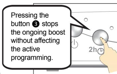
Pressing the button **3** stops the ongoing boost without affecting the active programming.
