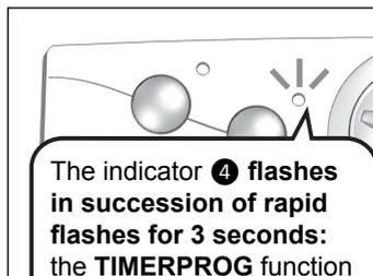
The indicator **4** flashes in succession of rapid flashes for 3 seconds: the **TIMERPROG** function is activated.
