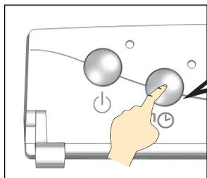
Press and hold the **3** button for **5 seconds**: the manual boost starts and time is recorded.
