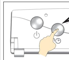
Press and hold the **3** button for **5 seconds** during a boost (manual or programmed).
