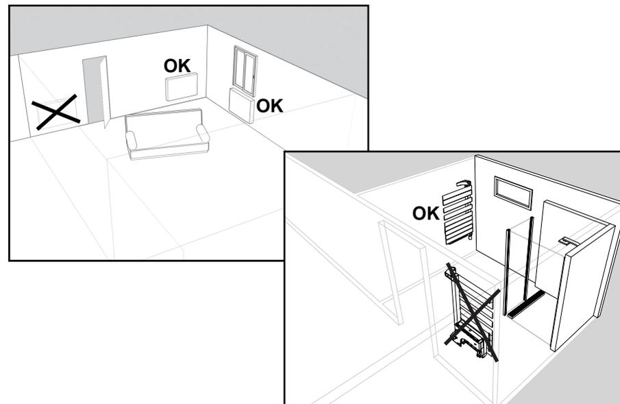
After opening a window, your appliance should detect the associated temperature drop within a reasonable period. It will then switch automatically to freeze protection mode (**7°C**). In this case the functioning indicator ❹ **flashes orange**.
