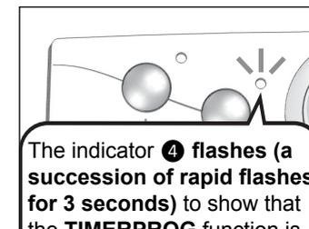
The indicator **4** **flashes (a succession of rapid flashes for 3 seconds)** to show that the **TIMERPROG** function is deactivated, and the current boost is stopped.
