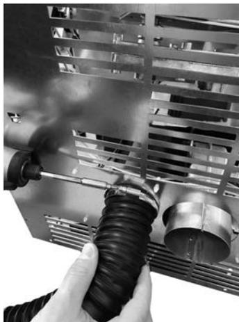
**Fig. 8 - Raccordement air comburant**
