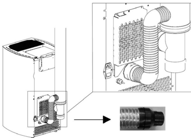
Fig. 11 - Tuyau flexible
