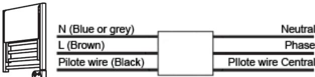
Configuration in which the pilot wire is not used.
