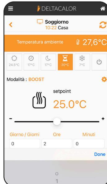
When the mode is enabled, the display alternates between the temperature measured in the room and the time left. Once the time has elapsed, the thermostat goes back to the last mode used.
