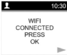
Once the screen shown here appears on the thermostat, the Wi-Fi configuration has been completed successfully and you now need to set the date and time. Press **OK** to proceed.
