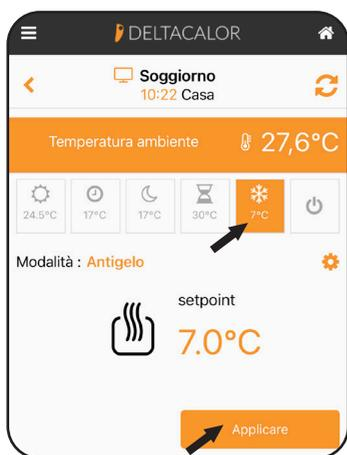
This mode enables you to set the thermostat to a non-modifiable temperature that protects the installation against freezing (7°C). To enable this mode, click the ❄️ icon and then click “Apply”.
