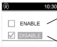
Select **enable** using the + and — keys. Press **OK** to enable ITCS.
