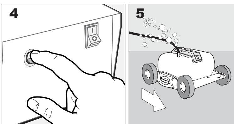
**EN** The Power-Control shuts OFF automatically when the cleaning cycle is completed.
