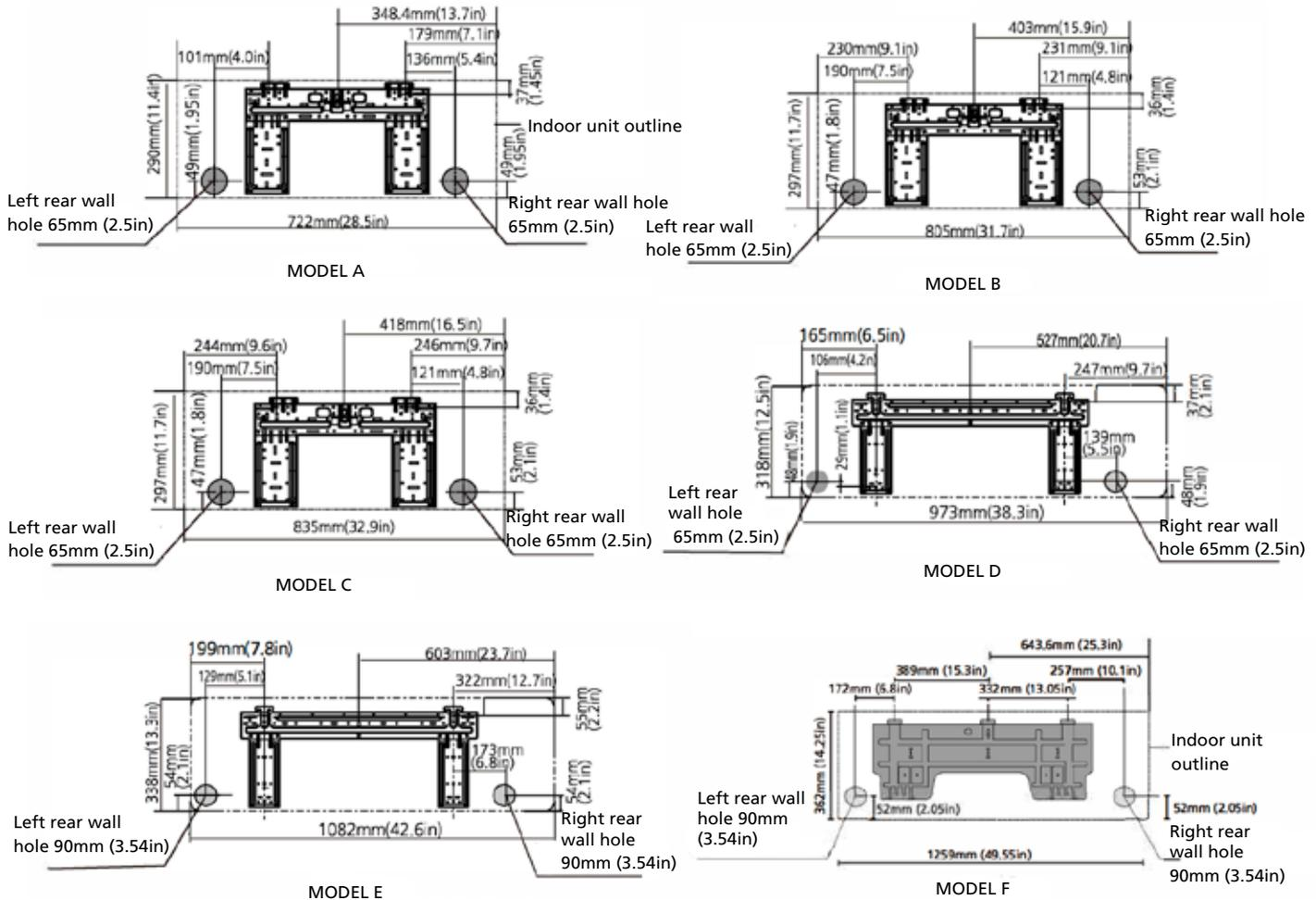
**NOTE:** When the gas side connective pipe is  $\Phi$  16mm(5/8in) or more, the wall hole should be 90mm(3.54in).
