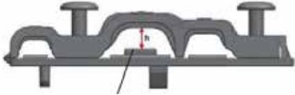
When the cable is not fasten enough, use the buckle to prop it up , so it can be clamped tightly.
