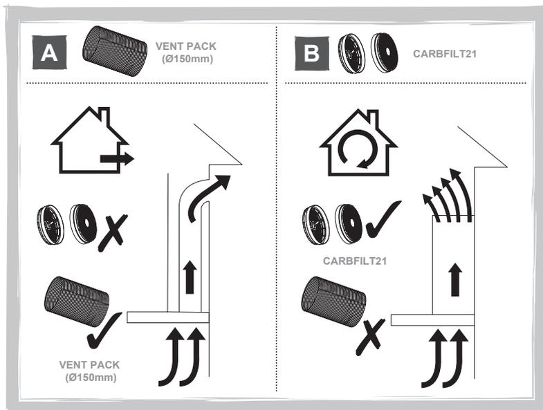
EN Choose a type of installation: Ducted option **A** (extraction to the outside) or Recirculation option **B** (no extraction to the outside). This appliance is for installation to a wall only.
